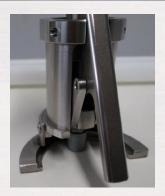
The Steinfurth Can Pressure Tester is easily ergonomic attached to beverage cans. It pierces eccentric the top lid of the can (for proper piercing outside of the pull ring area). The internal headspace can pressure can be read from the digital or analogue pressure gauge attached to the CPT piercing mechanic.
