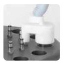
Chemically-resistant Easy-Or PTFE caps feature push-on connections to the stainless steel gas outlets.
