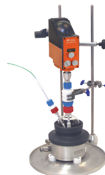
Breeze with 250ml Heat-On, stand and overhead stirrer
