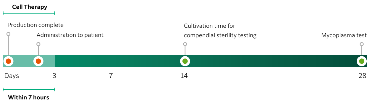
Figure 1. In the USP <71> Sterility Tests and Ph. Eur 2.6.1 Sterility, a 14-day incubation period is required. Regarding rapid test methods, the USP <1071> Rapid Microbial Tests and Ph. Eur. 5.1.6 Alternative Methods for Control allow for the use of rapid methods as alternatives and outlines important considerations for rapid tests.
