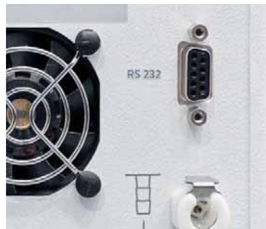
Standard-issue RS 232 interface for system integration into processes
