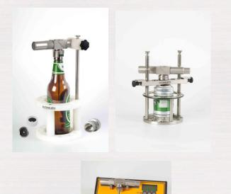
The Steinfurth PastControl system simplifies this task. The safe and simple operation requires only a short instruction to the operation personnel. The PU value can be read from the PU monitor's display directly at the pasteuriser line.
