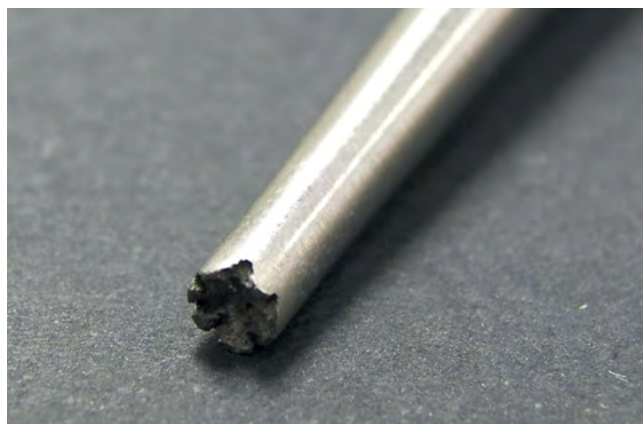
Example of a probe with cavitation erosion
