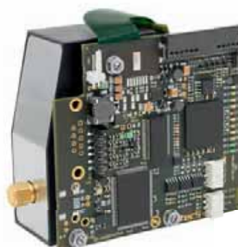
[SEU-CGS – Compact Electronics for Carl Zeiss CGS-CCD Spectral Sensor]
